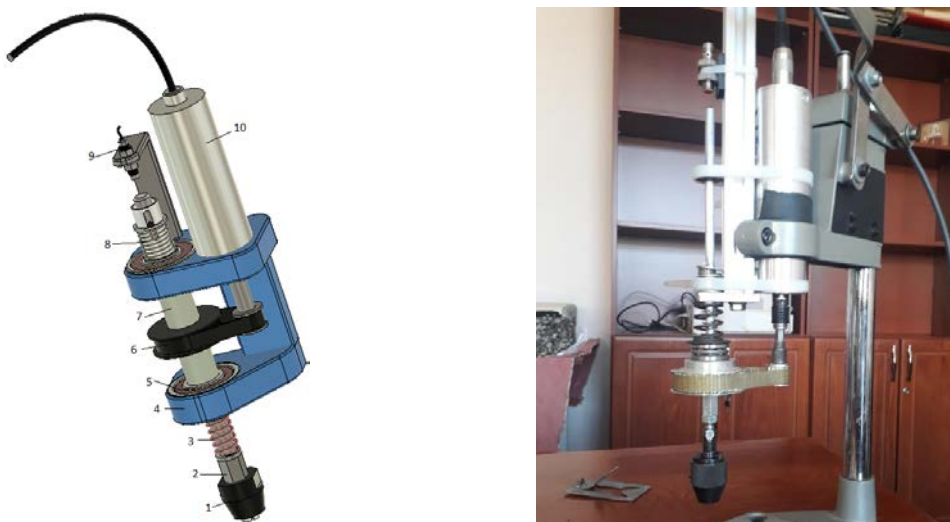
Figure 5. A 3D CAD model and the original model tool for capacitors' dismantling 1 – mandrel; 2 – mandrel sliding spindle; 3 – clamping spring; 4 – device support; 5 – bearings; 6 – gears assembly with belt connection; 7 – rotation shaft; 8 – supporting mobile spring in the workspace with limited backlashes values; 9 – proximity capacitive sensor with a continuous adjustment possibility; 10 – a programmable screwdriver
