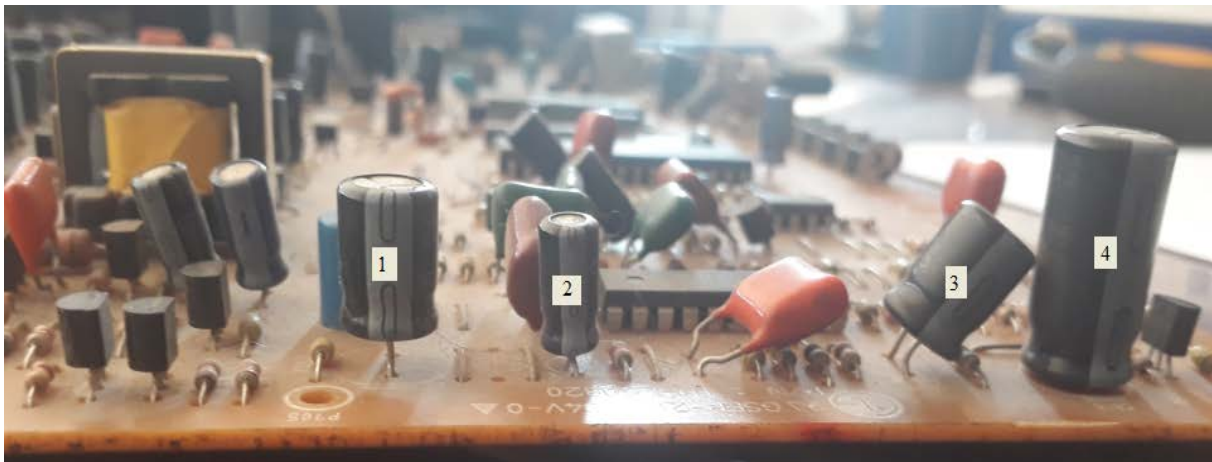
Figure 6. Different attachment ways for capacitors to the PCB 1,3 – longer pins and 2, 4 – smaller pins
