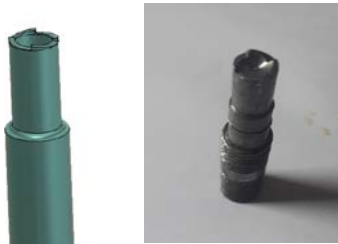
Figure 4. A CAD design and a real mandrel type tool with saw teeth for capacitors dismantling
