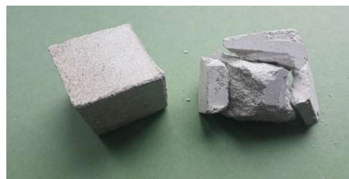
Fig. 2. Stone sample before and after mechanical testing
